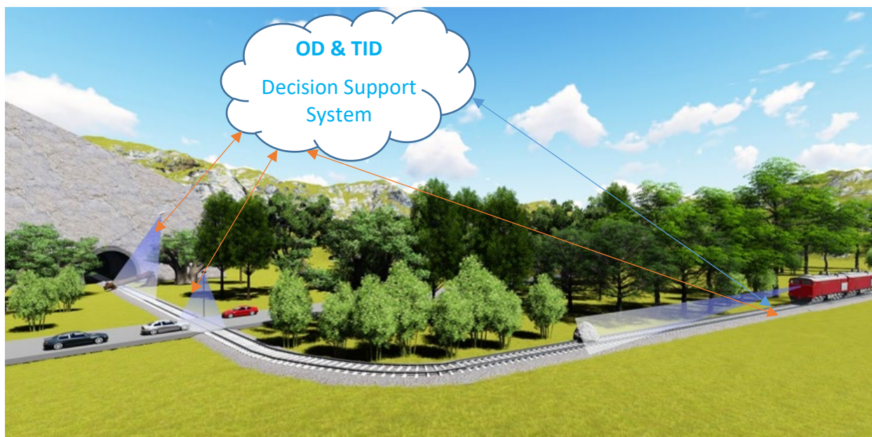
Figure 10: Concept of SMART2 holistic system for OD& TID consisting of on-board, trackside and drone-based OD& TID sub-systems, interfacing with central DSS unit
