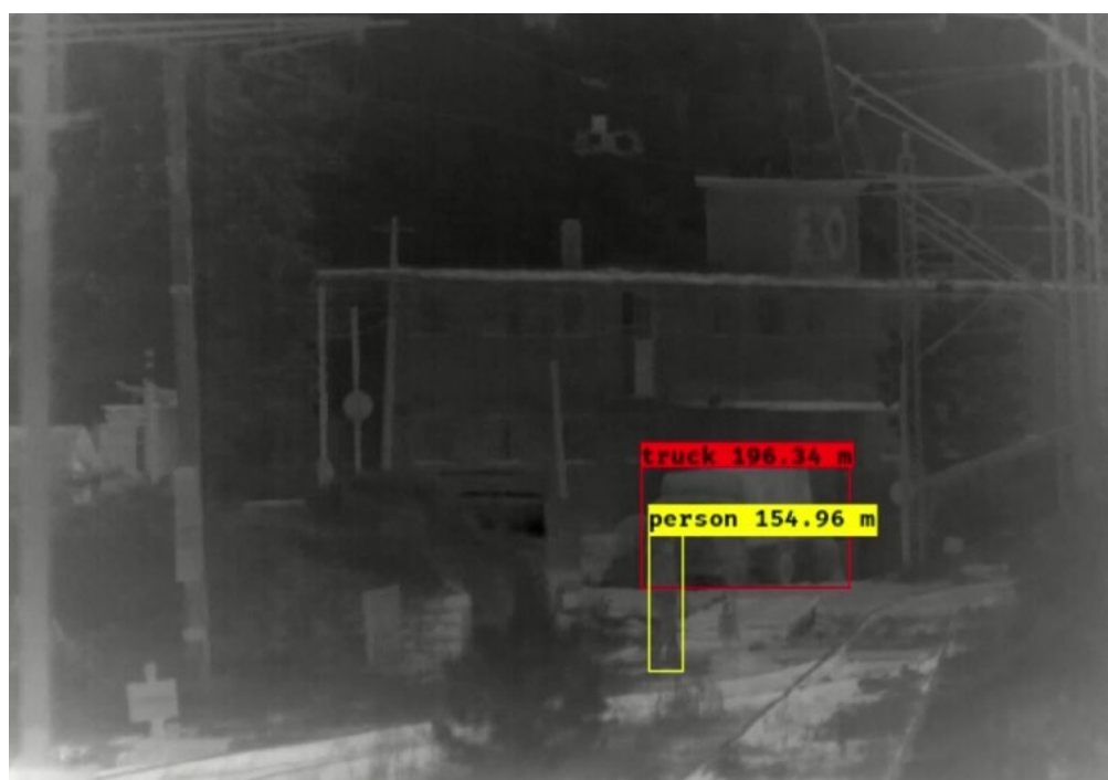
Figure 7: Object detection and distance estimation in on-board thermal camera image recorded in environmental condition of 38°C; Good detection result despite low-contrast image; Ground truth distance for person: 155 m (error 0.025 %) (SMART, 2019)
