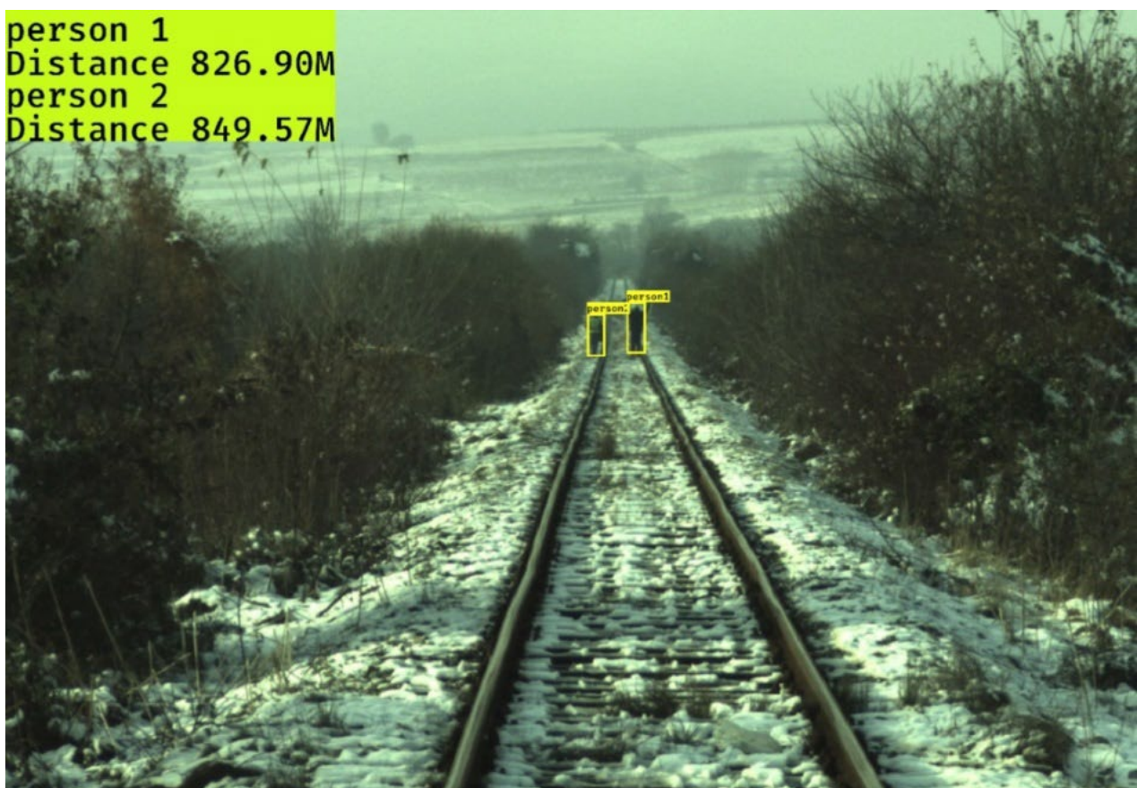
Figure 5: Object detection and distance estimation in RGB camera image recorded in winter (snow) environmental conditions; Ground truth distance: 835 m (distance estimation error for person 1 and person 2 was 0.97 % and 1.74% respectively) (SMART, 2019)
