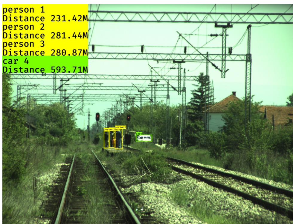
Figure 6: Object detection and distance estimation in on-board RGB camera image; Ground truth distance: for persons (station middle point) 266.69 m (average error 8.32%), for the car 597.87 m (error 0.69%) (SMART, 2019)
