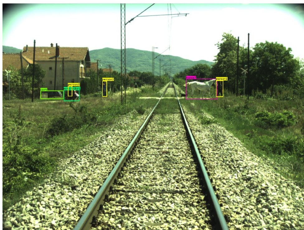
Figure 9: Object classification in real-world scene: persons and an animal (horse) are crossing the rail tracks on unsecured crossing while train is approaching; Person on the motorbike is “waiting” on the left side of the rail tracks crossing and a car is parked on the left side of the rail tracks (SMART, 2019)
