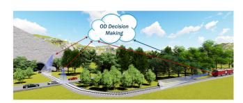
In SMART2, the on-board OD system is complemented by UAV-based and trackside OD systems to increase the detection area.
